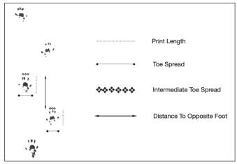
Figure 1: SFI parameters from rat footprints obtained from the walking corridor.
