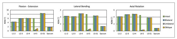
Figure 2: Comparison of the global range of motion (degree) of uninstrumented spine and three rod configurations (bilateral, oblique and unilateral) under flexion-extension, lateral bending and axial rotation.
