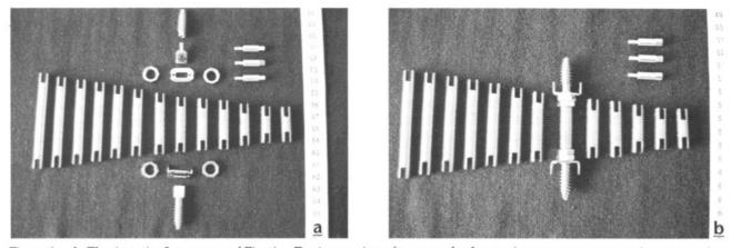
Figure 1, a, b: The Anterior Intercorporal Fixation Device consists of two standard spongious screws, two rotation preventing washers, a connector, and two connector fixing screws that connect the spongious screws to the connector.
