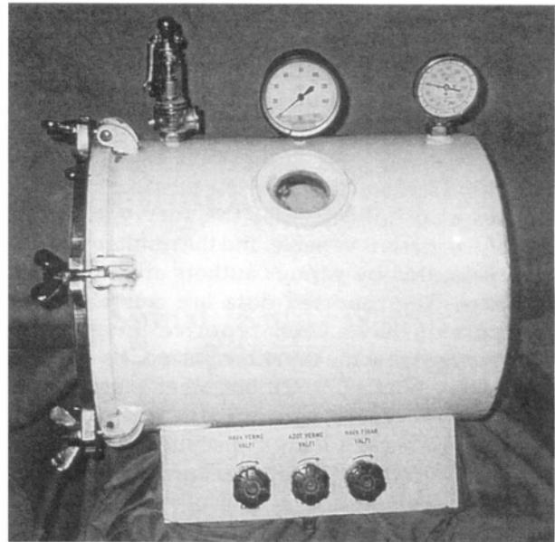
Figure 1: Photograph of the hyperbaric oxygen application chamber that was specifically designed for the experimental studies.
