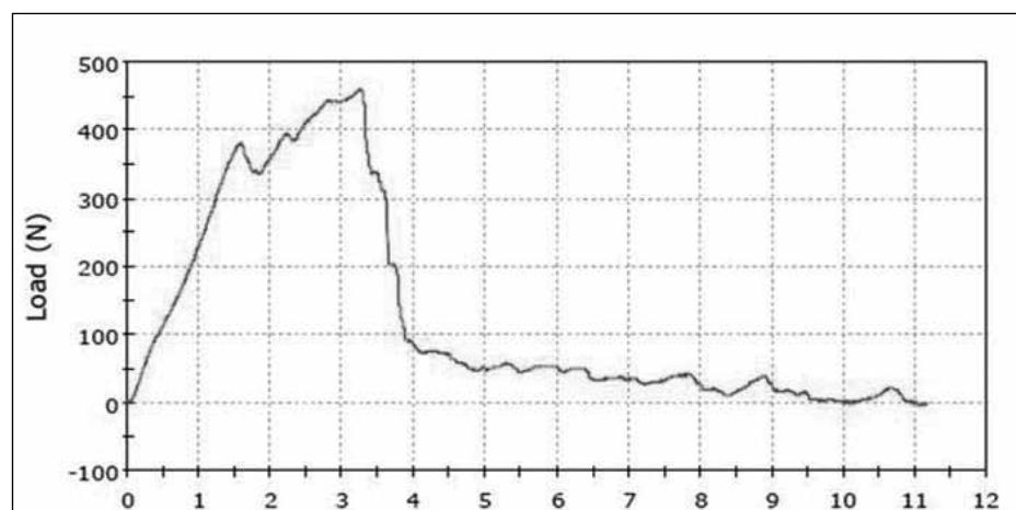
**Figure 4:** Graph showing pullout values of the screw without "Dubel". The peak pullout value was 456.09102 Newton for this specimen.
