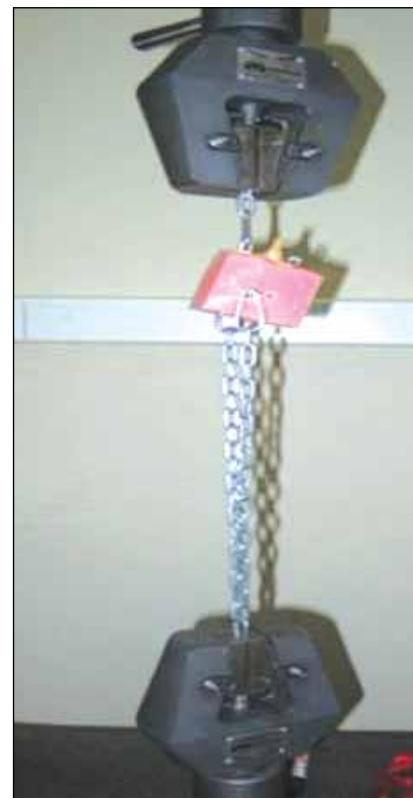
**Figure 3:** Pullout test of the specimen with the Instron 850 biomechanical testing machine.
