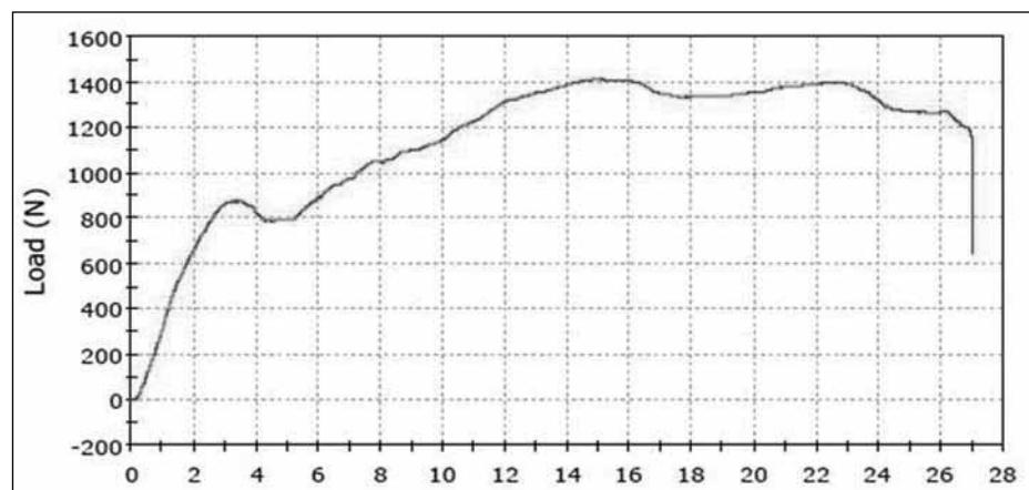
**Figure 5:** Graph showing the pullout values of screw with "Dubel". The peak pullout value for this specimen was 1408.33 Newton.
