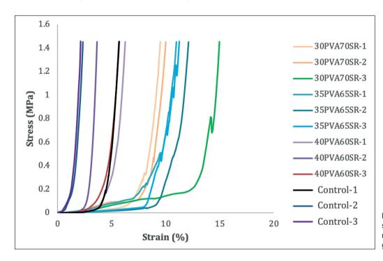
Figure 4: Stress (MPa) and strain (%) graph of the silicone rubber and PVA material group and control.
