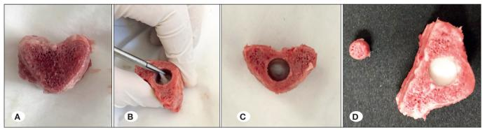
Figure 2: Specimen preparation of the lumbar vertebral body and intervertebral disc. A) Anterior column unit (ACU) of the lumbar vertebral body. B) Taking the nucleus pulposus. C) ACU without nucleus pulposus. D) ACU filled with the silicone rubber and PVA material.
