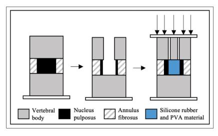
Figure 3: Compressive mechanical testing procedure.
